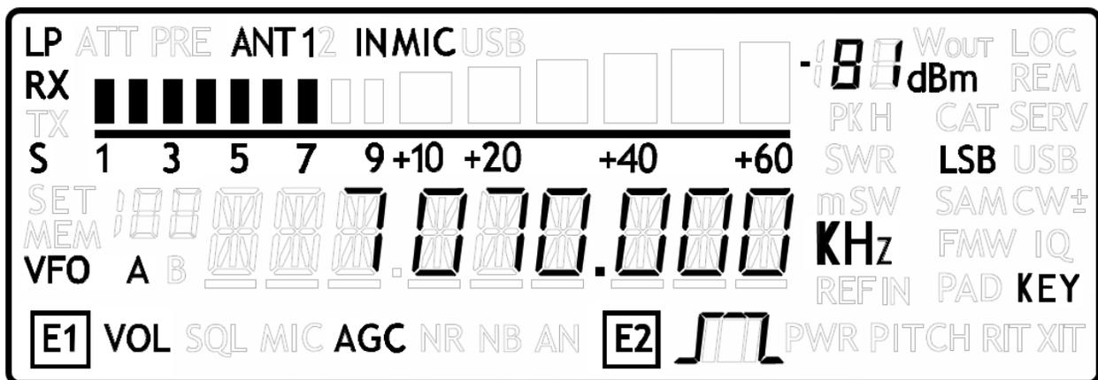
After some seconds the device is in reception mode with VFO A enabled.
