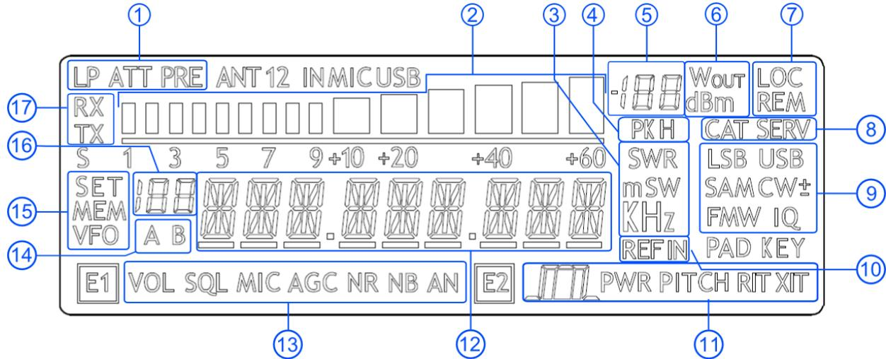
1. LP: turns on when the low pass filter is active.
