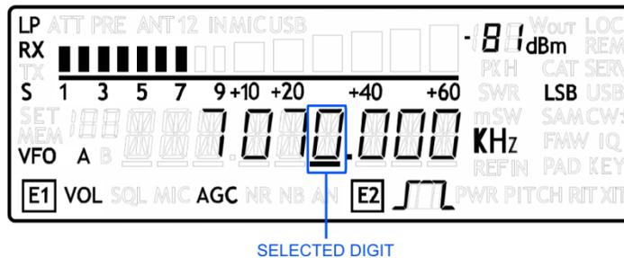
In this mode use the main knob to modify the selected digit and E1 or E2 to change witch digit you want to modify. Apply a short pressure on main knob to return in the standard tuning mode.
