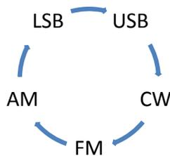
When you do not use the FM mode, you can disable it with the setting menu 14 “FM MODE”. The main purpose of this functionality is to not hear the FM exasperating noise when changing between modes and you are not using the FM mode.
