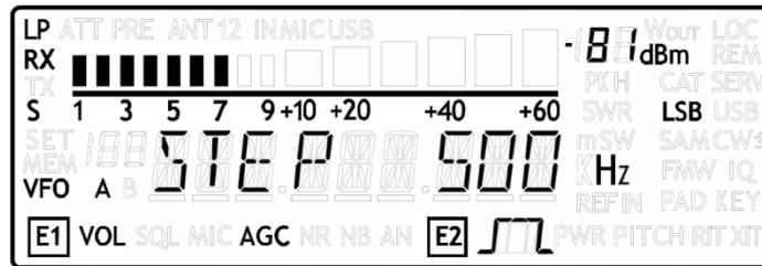
Use the main knob to modify the tuning step, then with a short pressure return in the VFO menu.
