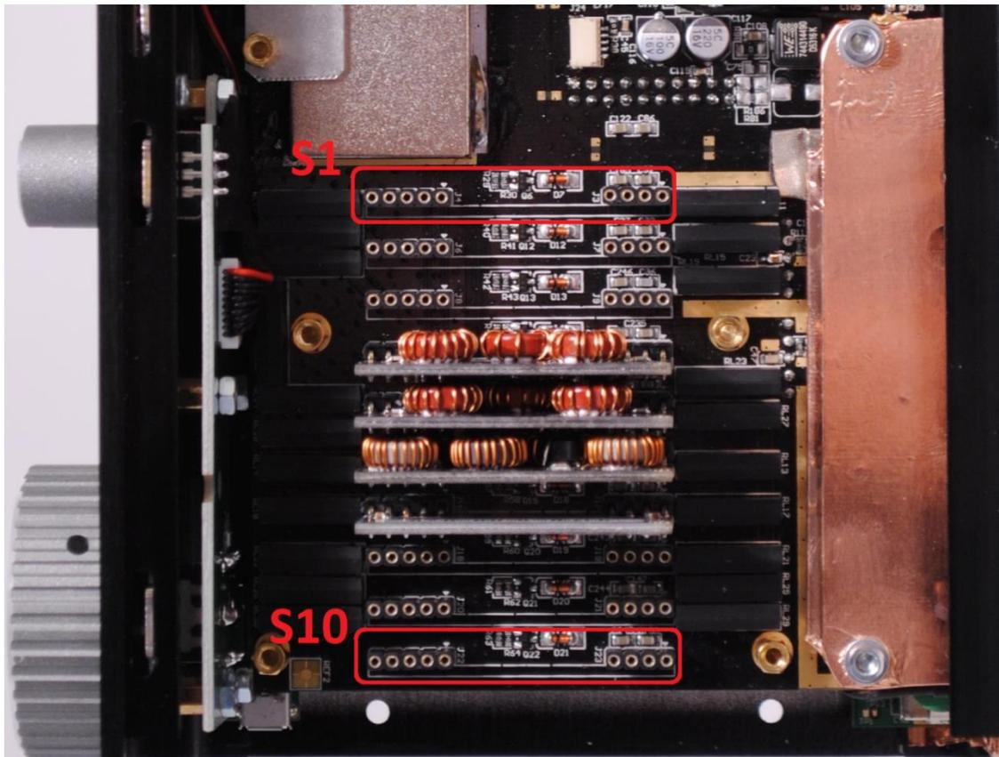
As shown in the FDM-DUOr front end block diagram below, use slots 4 to 10 for HF (under Antenna 1) and slots 1 to 3 if using Antenna 2 (no low pass filter).
